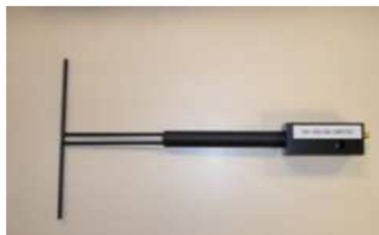
Figure 1 – Satimo COMOSAR Validation Dipole
