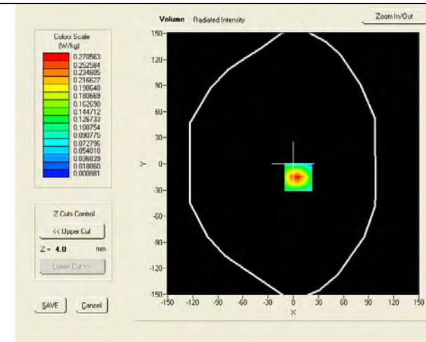
**SAR, Z Axis Scan (X = 6, Y = -15)**
