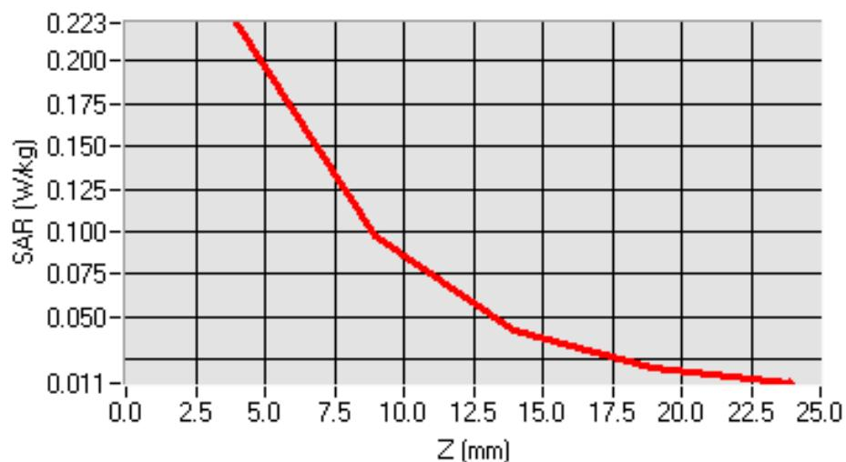
Test mode: GSM1900, Low channel (Left Head Tilt)
