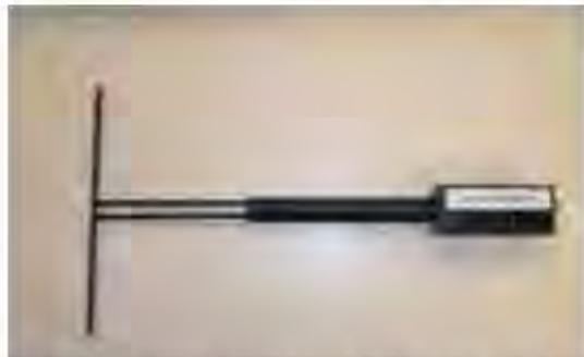
Figure 1 – Satimo COMOSAR Validation Dipole
