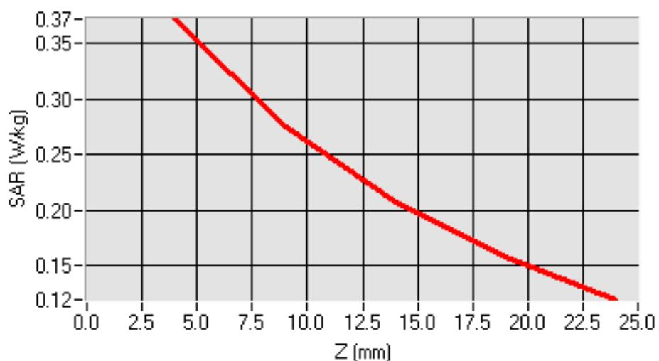
Test mode: GPRS850, low channel (Body-LCD DOWN)
