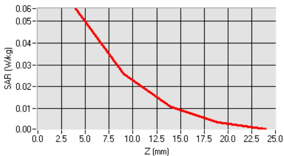
Test mode: GPRS1900, Low channel (Body LCD-UP)
