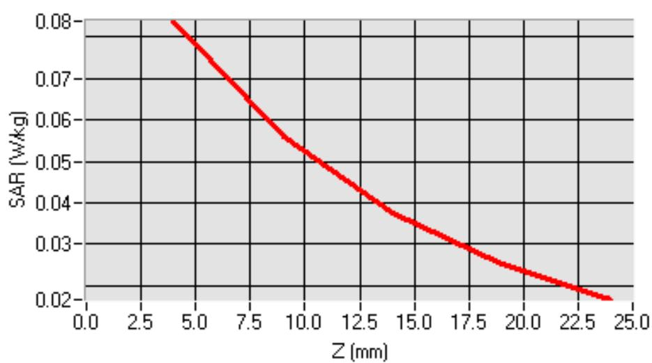
Test mode: GSM1900, Low channel (Left Head Cheek)
