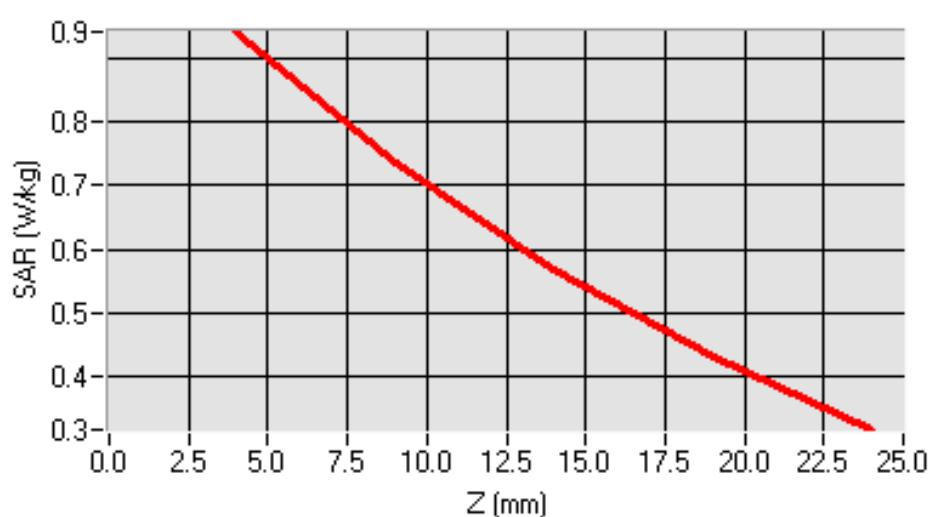
Test mode: GSM1900, Low channel (Right Head Cheek)
