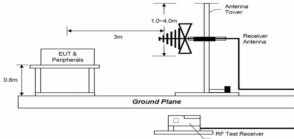
**Radiated Emission Test Set-Up, Frequency above 1GHz**
