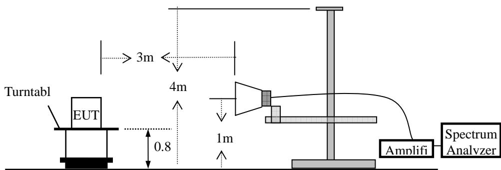
**Substituted Method Test Set-UP**
