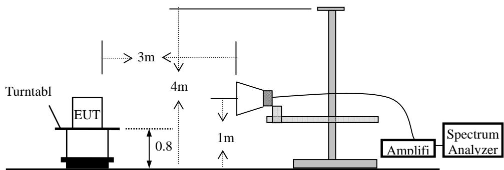
**Substituted Method Test Set-UP**
