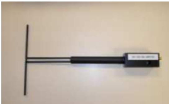
Figure 1 – Satimo COMOSAR Validation Dipole
