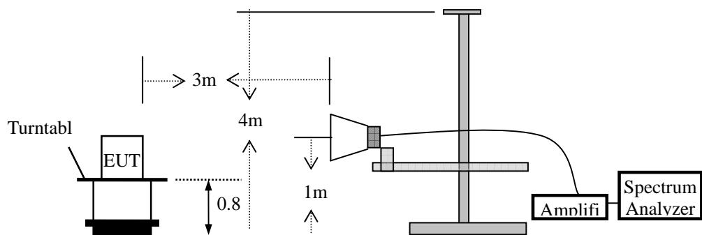
**Substituted Method Test Set-UP**
