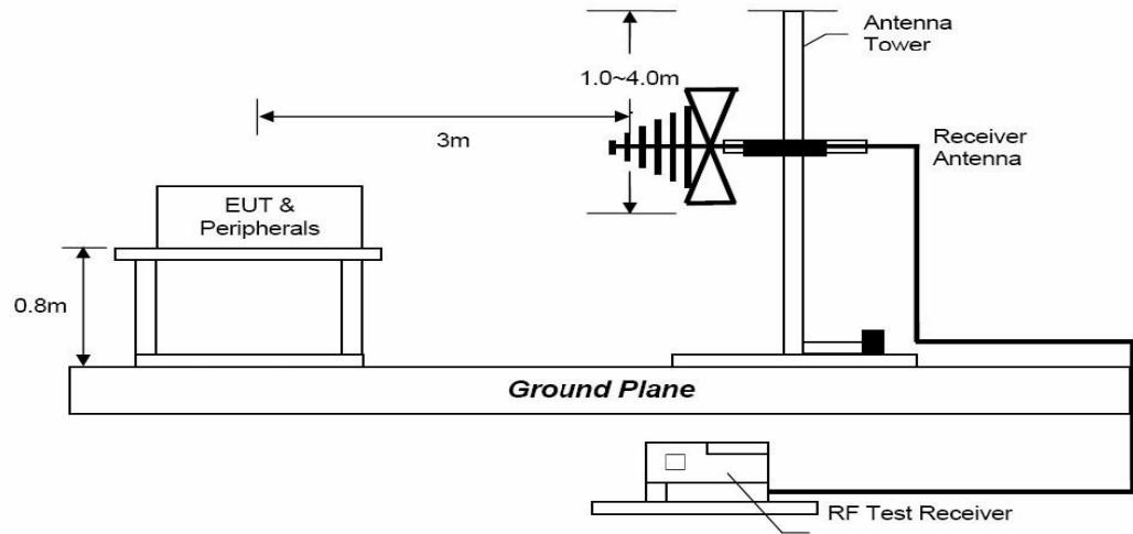
**Radiated Emission Test Set-Up, Frequency above 1GHz**
