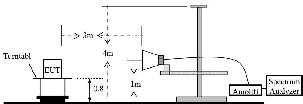
**Substituted Method Test Set-UP**
