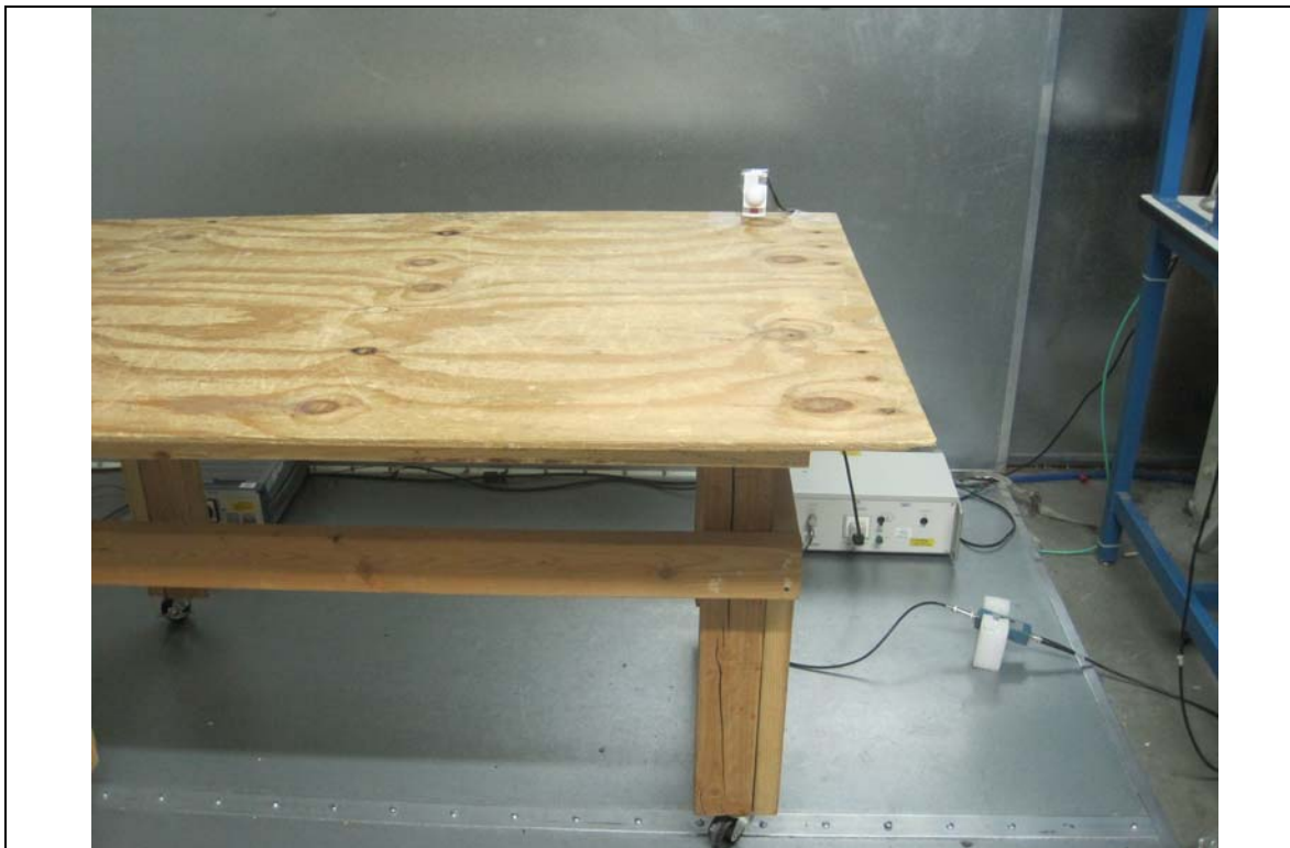
Conducted Emission Test Setup – Front View
