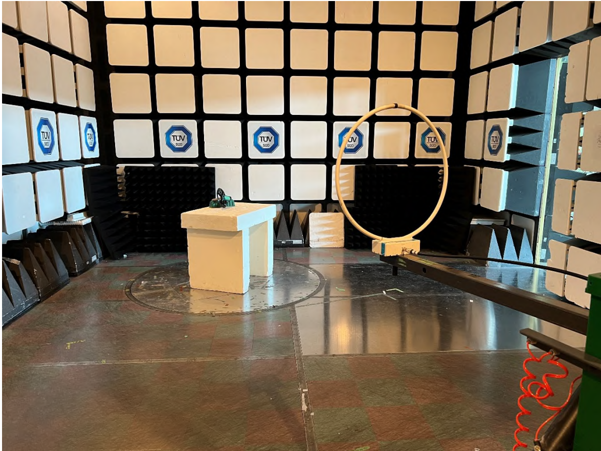
Figure 10 – Radiated Emissions Setup 9kHz – 30MHz
