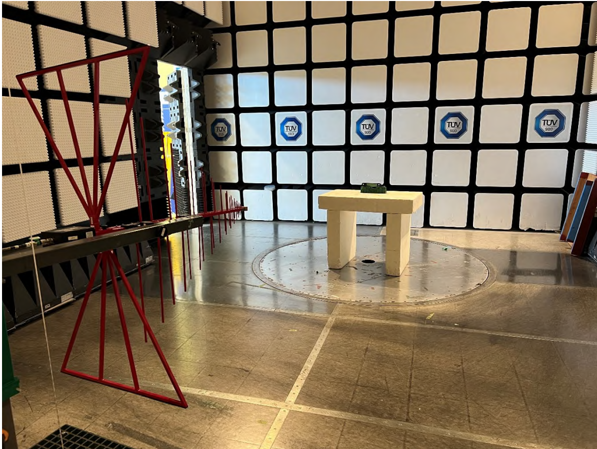
Figure 3 – Radiated Emissions Setup 30MHz – 1GHz
