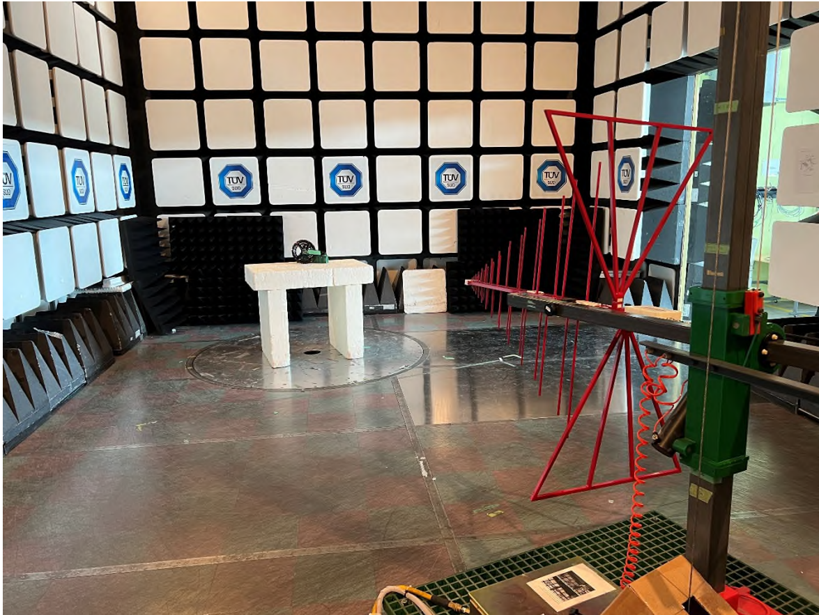
Figure 11 – Radiated Emissions Setup 30MHz – 1GHz
