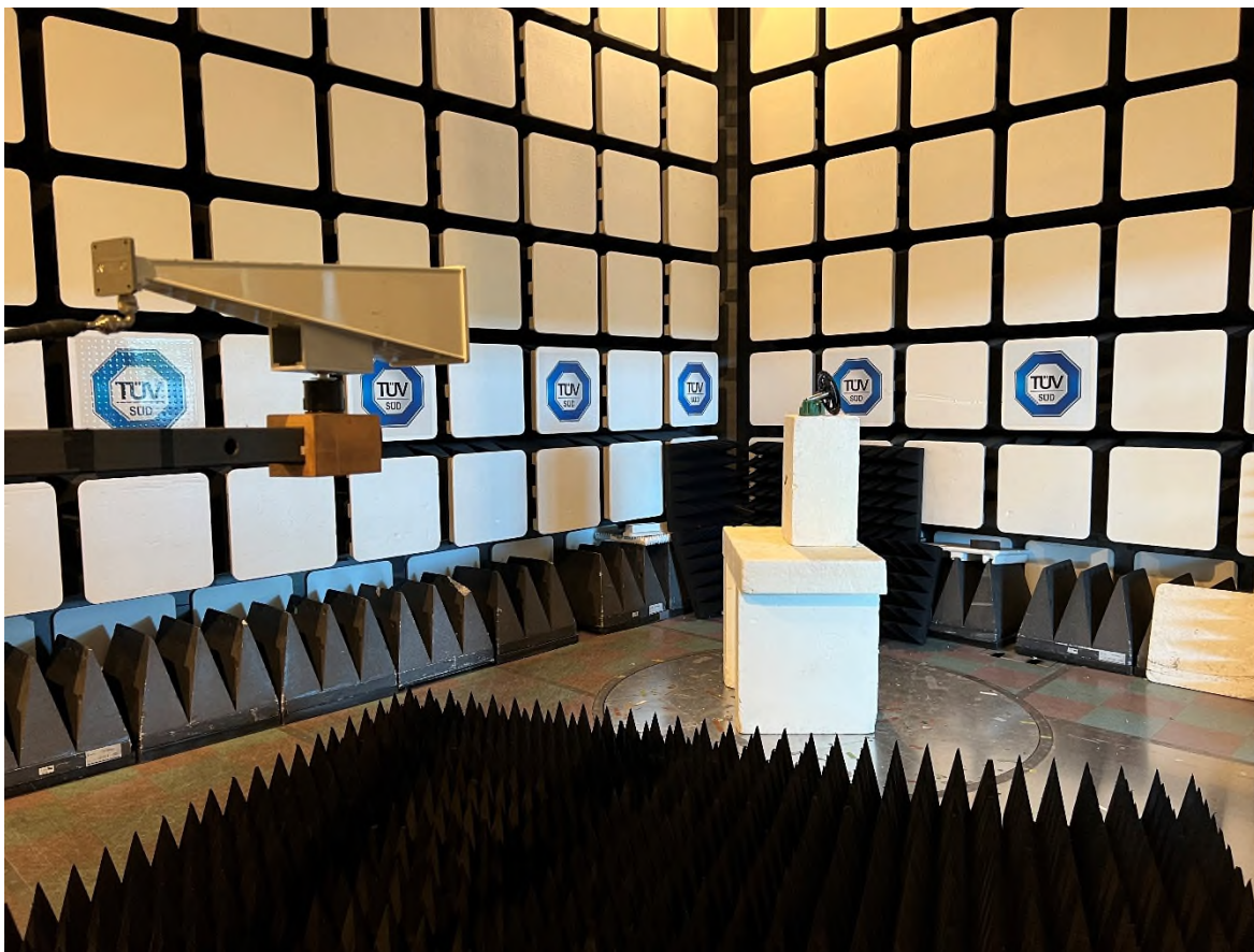
Figure 13 – Radiated Emissions Setup 6GHz – 10GHz
