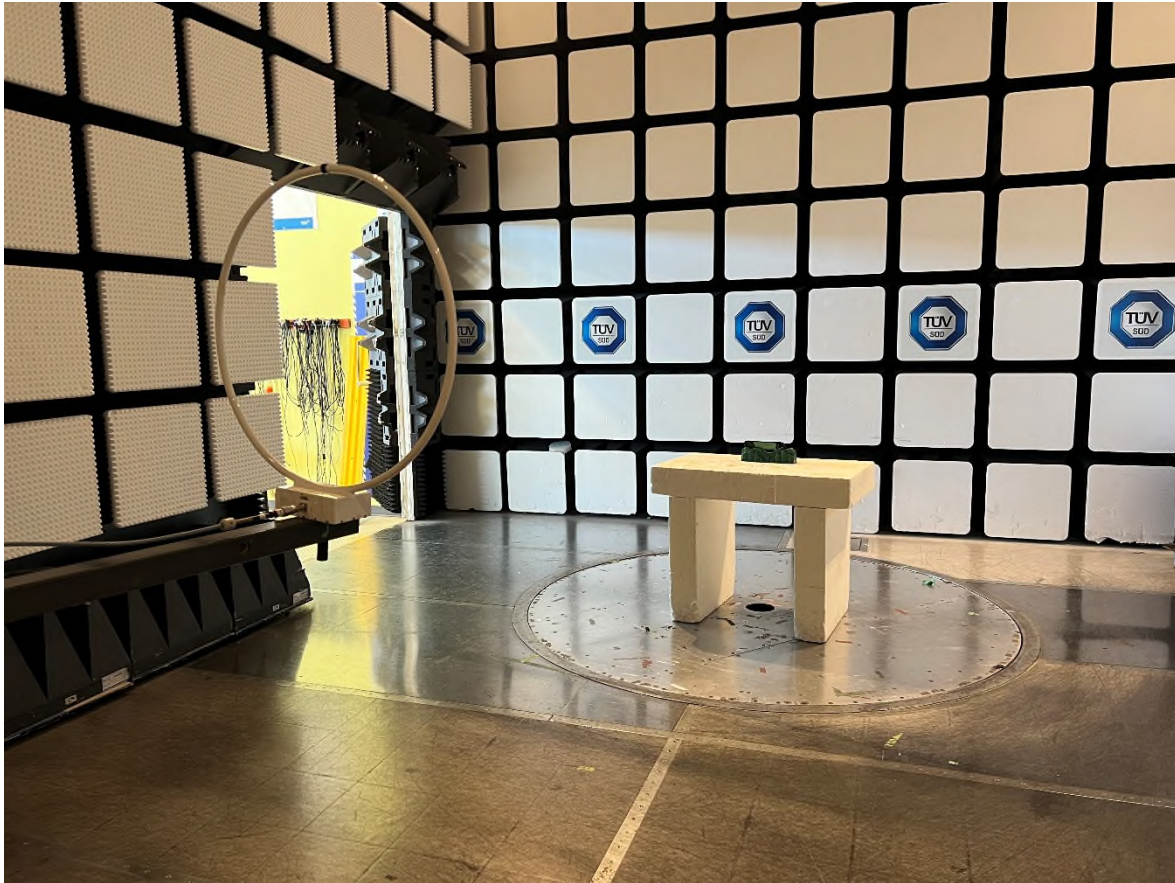
Figure 2 – Radiated Emissions Setup 9kHz – 30MHz
