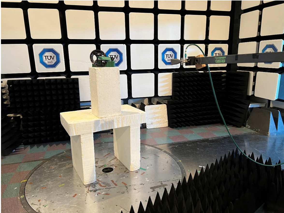
Figure 15 – Radiated Emissions Setup 18GHz – 25GHz
