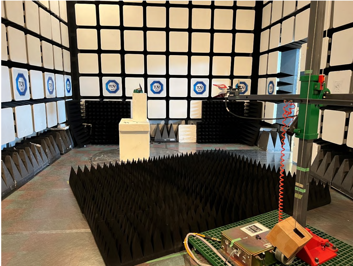
Figure 12 – Radiated Emissions Setup 1GHz – 6GHz
