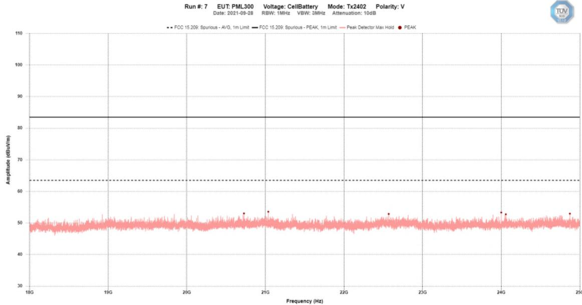
Plot was taken at a 1 meter distance. All emissions were noise floor of measurement instrument. No emissions were found in this frequency range.
