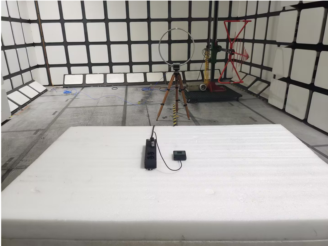
Radiated Emissions View (Below 1 GHz)
