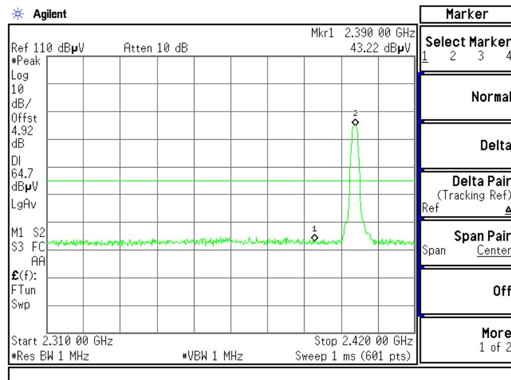
**Band Edges (CH High)****Detector mode: Peak****Polarity: Vertical**
