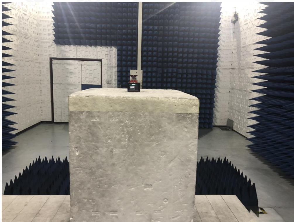
FCC RADIATED EMISSION TEST SETUP ABOVE 1GHZ
