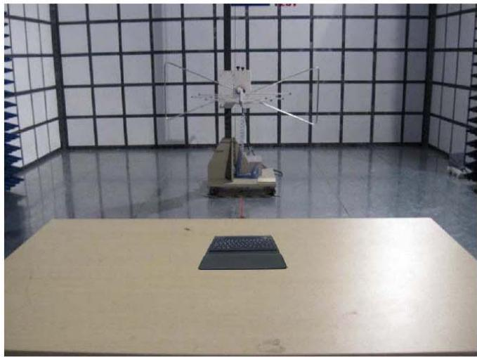
**Radiation Emission Test Setup**
