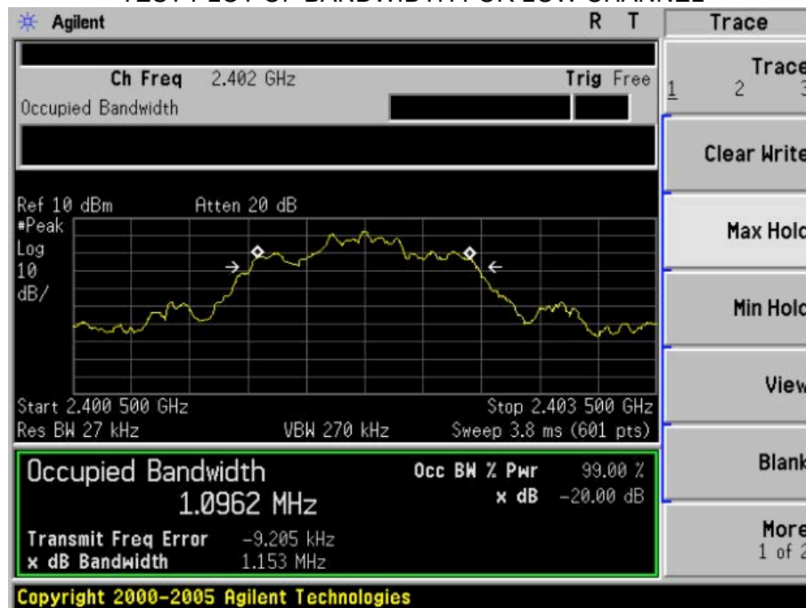
TEST PLOT OF BANDWIDTH FOR LOW CHANNEL
