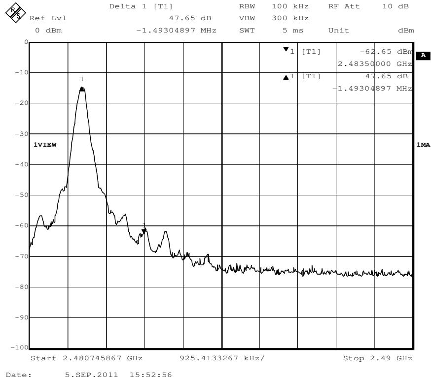
For 2.4835 GHz bandage checked with 2.482 GHz frequency operated, the delta shown at the plots are -47.65 dB for peak detector mode.
