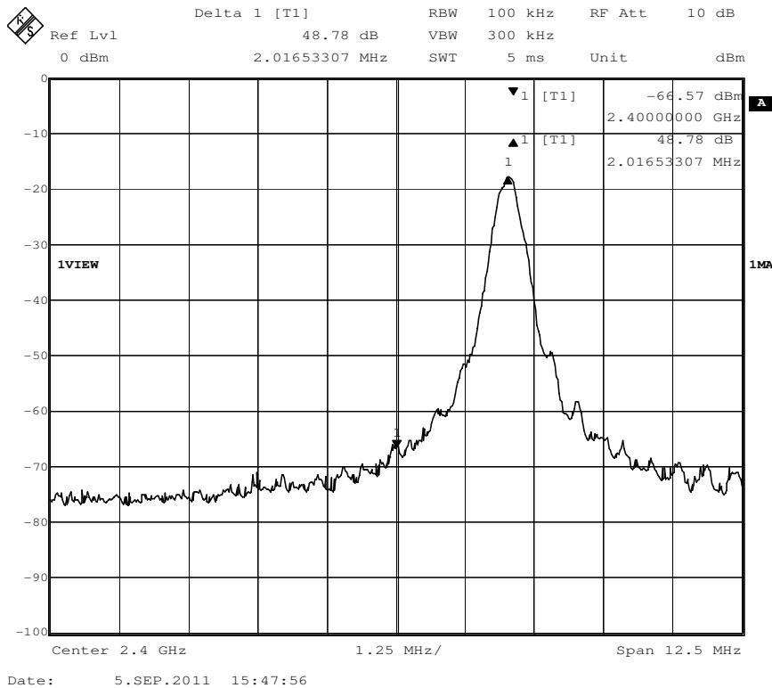
For 2.400 GHz band edge checked with 2.402 GHz frequency operated, the delta shown at the plots are -48.78 dB for peak detector mode
