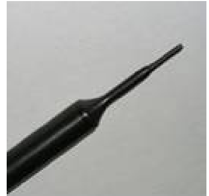
Figure 2. EX3DV4 E-field Probe
