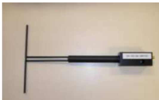
Figure 1 – Satimo COMOSAR Validation Dipole
