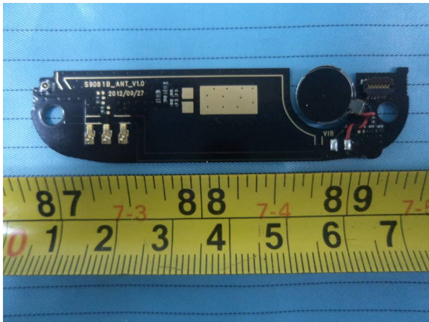
EUT – Antenna Board Top View
