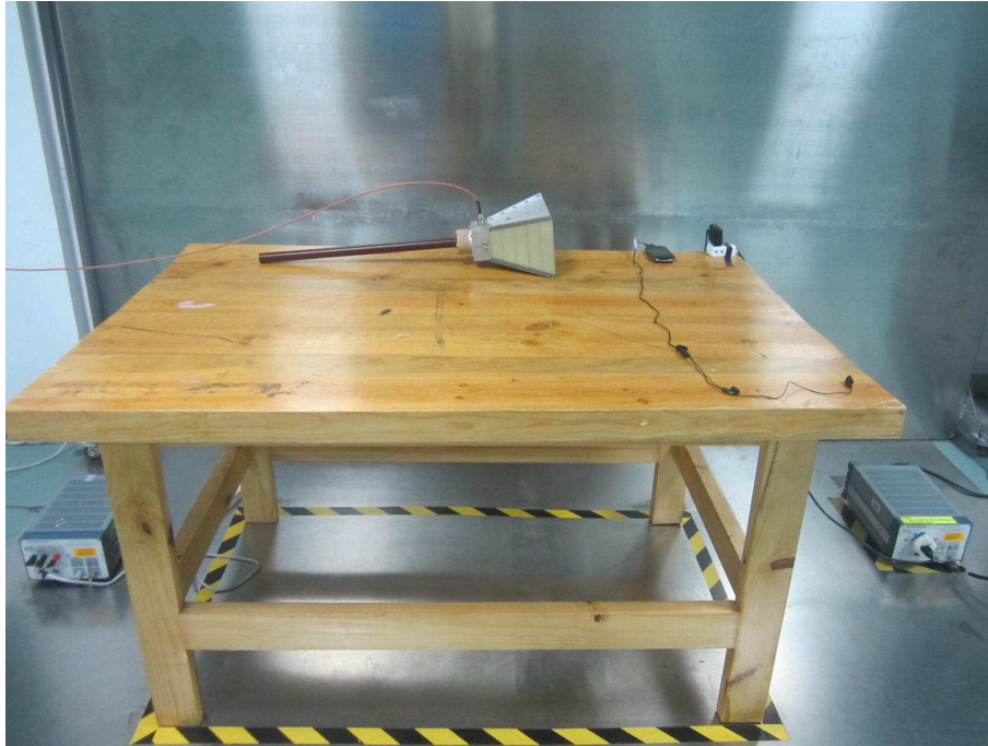
Conducted Emission - Side View
