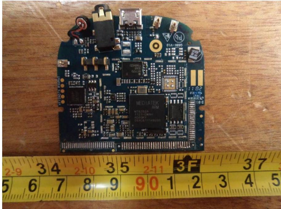
**EUT – RF Board 1 Bottom View**
