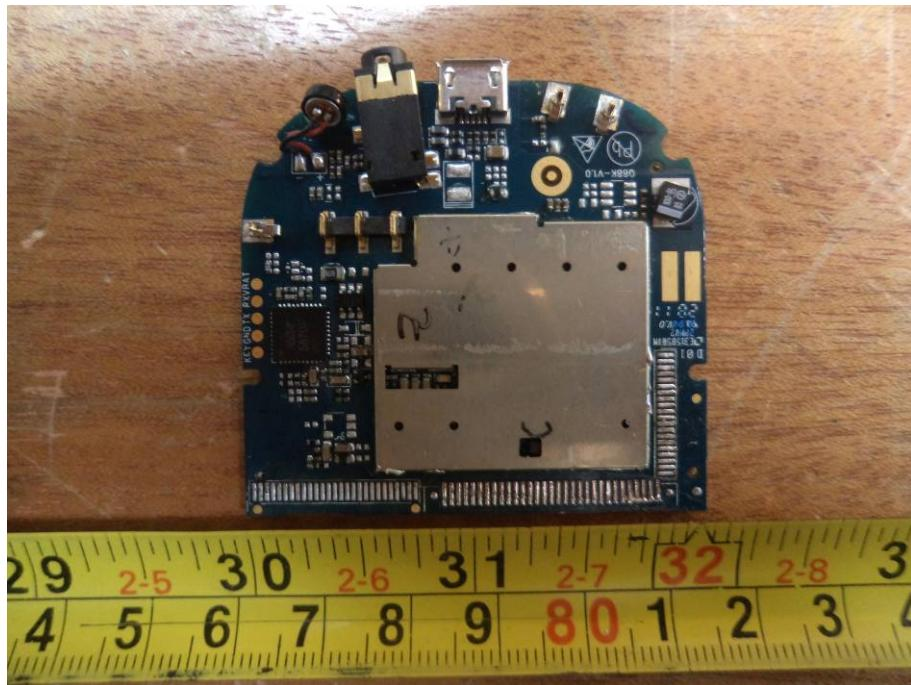
**EUT – RF Board 1 Top Shielding off View**
