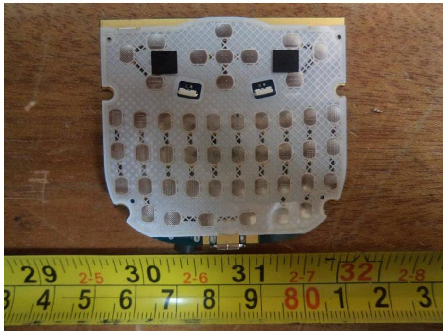
**EUT – RF Board 2 Top View**
