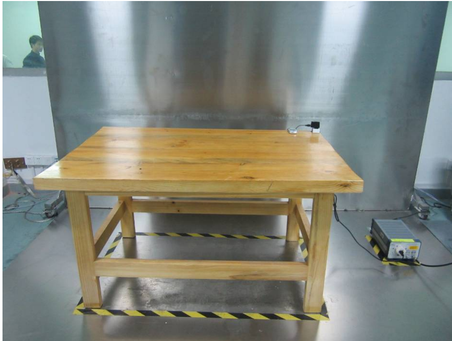
Conducted Emissions - Side View (Charging mode)
