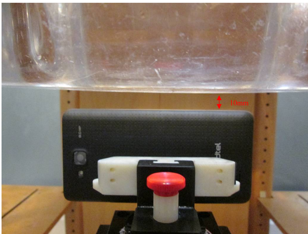
Body-worn Right Setup Photo (10mm)
