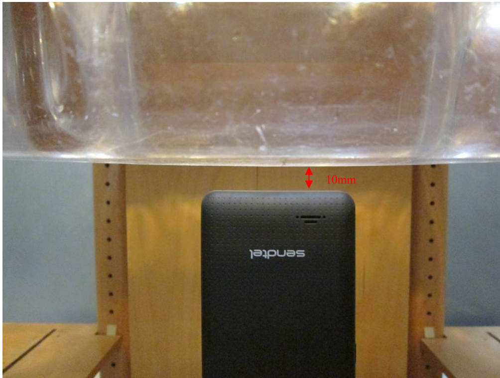
Body-worn Bottom Setup Photo (10mm)
