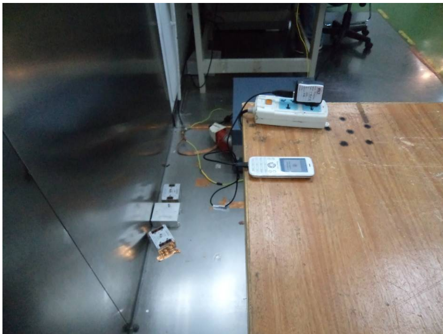
Conducted Emissions - Side View (Charging & media playing)
