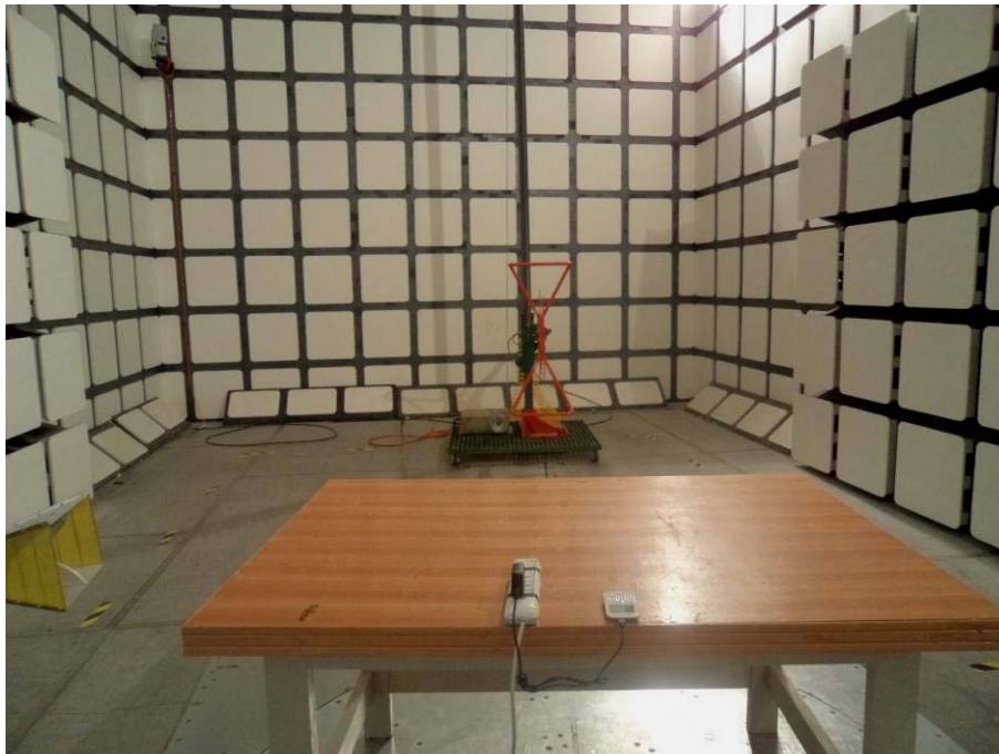
Radiated Emissions - Rear View (Charging & multimedia playing)
