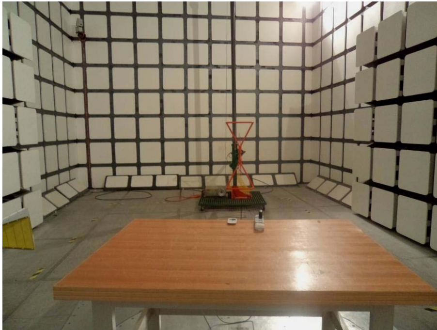
Radiated Emissions - Rear View (Charging & multimedia playing)
