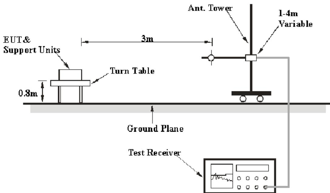
The radiated emission tests were performed in the 3 meters chamber B test site, using the setup accordance with the ANSI C63.4-2009. The specification used was the FCC 15.209, and FCC 15.247 limits.
