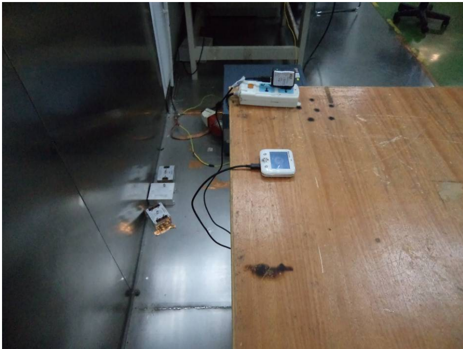
Conducted Emissions - Side View (Charging & Media Playing)
