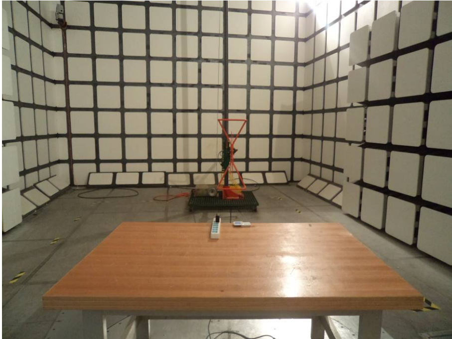
Radiated Emissions - Rear View (Charging & Media Playing)
