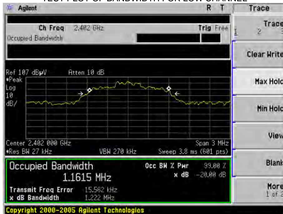
TEST PLOT OF BANDWIDTH FOR LOW CHANNEL
