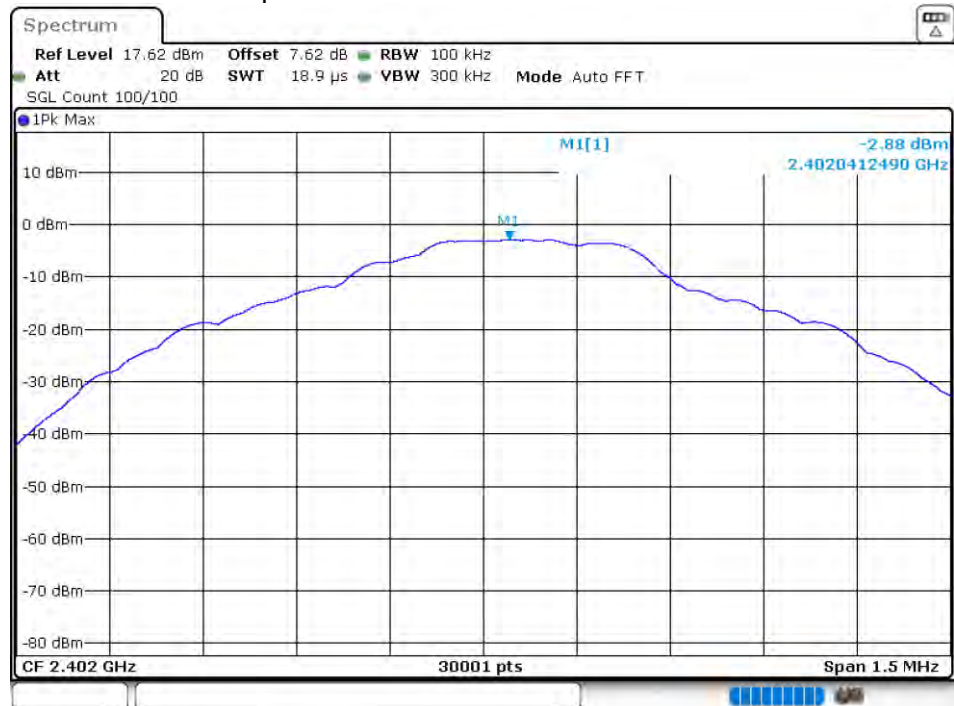
Tx. Spurious NVNT 1-DH5 2402MHz Ant1 Ref
