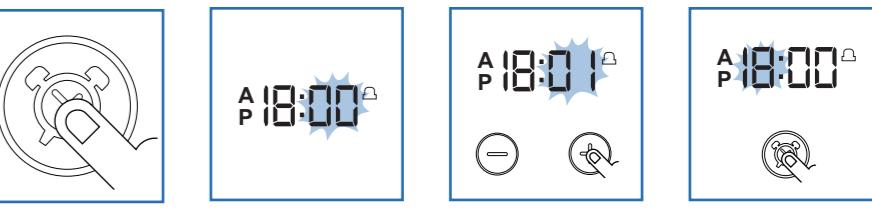
Long press the ALARM button to set alarm time minutes flash adjusted via pressing VOL +/VOL- button.
