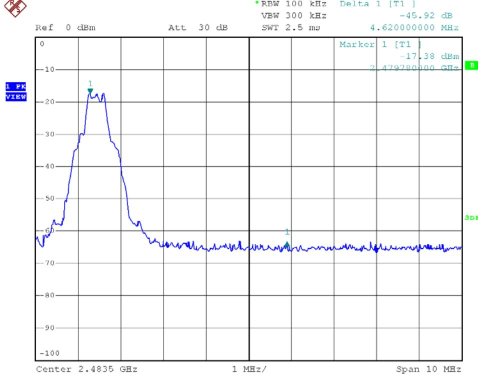
Bandwidth / Bandedge Plot – Pursuant to FCC Part 15 Section 15. 249 Requirement (Pass/Fail)
