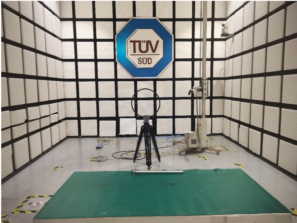
Radiated Emission Setup 9kHz ~ 30MHz
