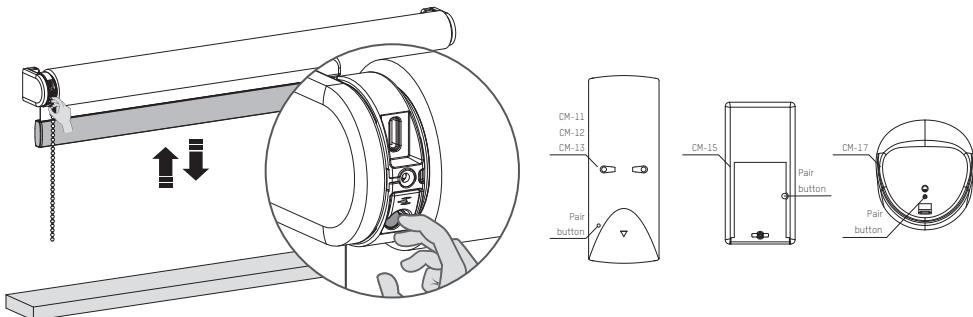
.2 Press the pair button on the back of the remote control to pair the blind with the selected channel. The blind will shortly stop stepping, indicating that the remote has been paired to the blind.
