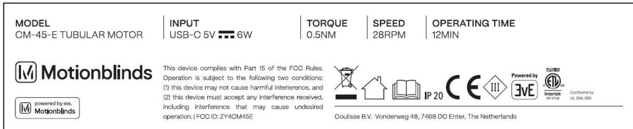
Specifications: The label shall be securely affixed to a permanently attached part of the device, in a location where it is visible or easily accessible to the user, and shall not be readily detachable. The label shall be sufficiently durable to remain fully legible and intact on the device in all normal conditions of use throughout the device's expected lifetime.
