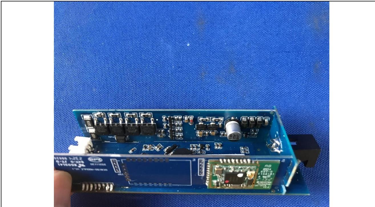
Details of: PCB view (433.925MHz module)
