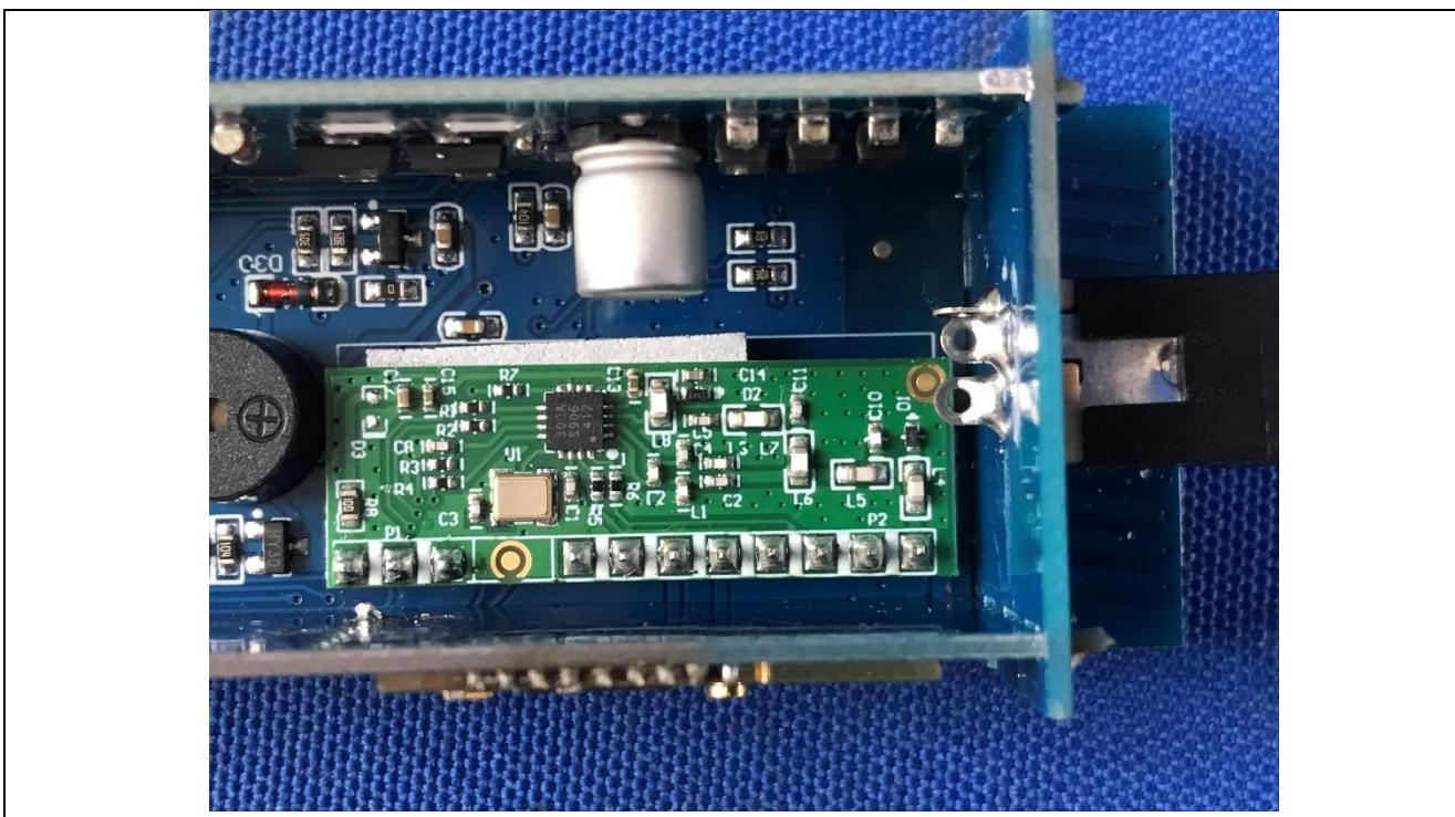
Details of: PCB view (BLE/Thread module)
