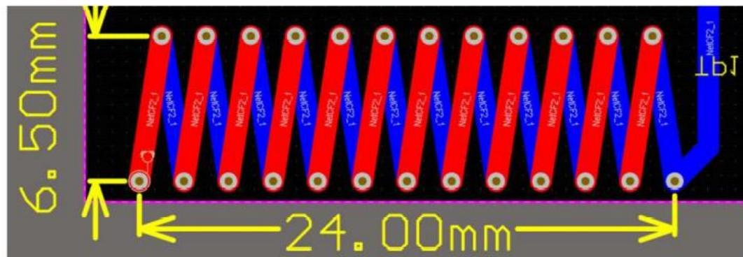
Antenna transmission frequency: 433.925MHz
