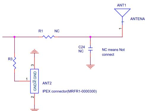
And the following antenna is connected to IPEX port while in use.
