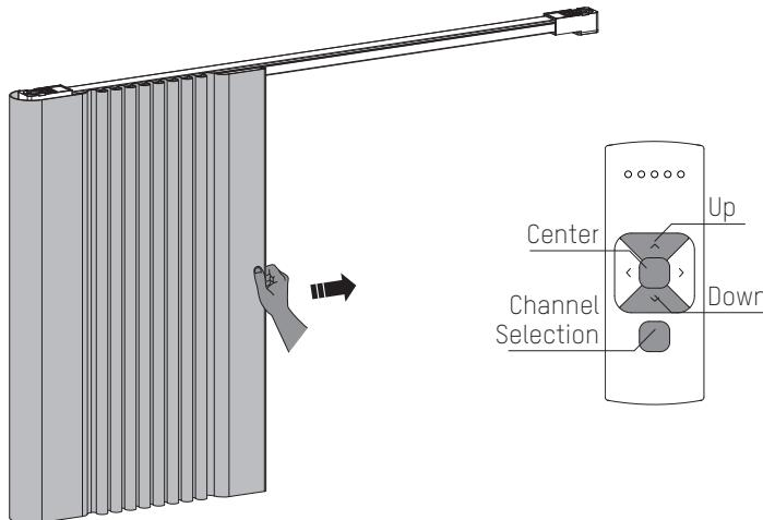
**i** Remote control: Choose the channel to which the blind has been paired using the channel button. Press the up or down button to operate the blind. Press the center button to stop the blind. Use the left and right button to move the blind in small steps.
