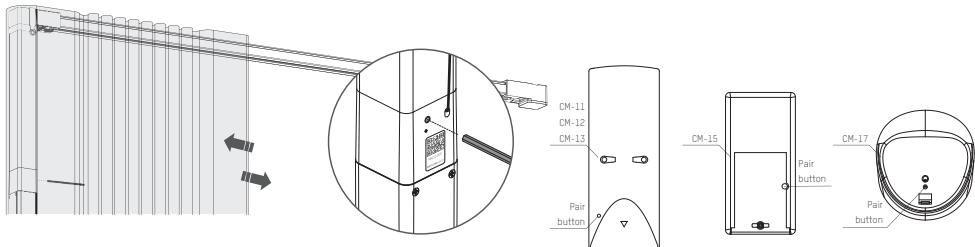
.2 Press the pair button on the back of the remote control to pair the blind with the selected channel. The blind will shortly stop stepping, indicating that the remote has been paired to the blind.
