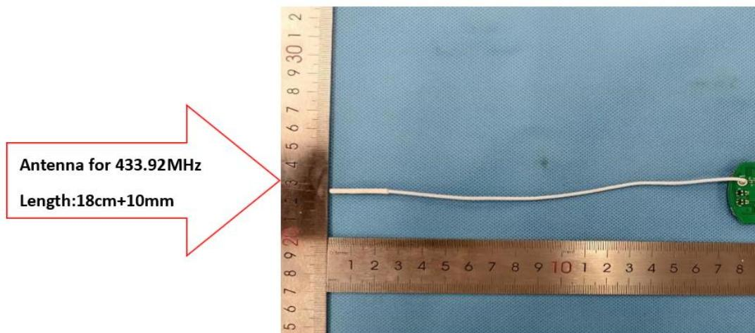
Antenna transmission frequency: 433.92MHz
