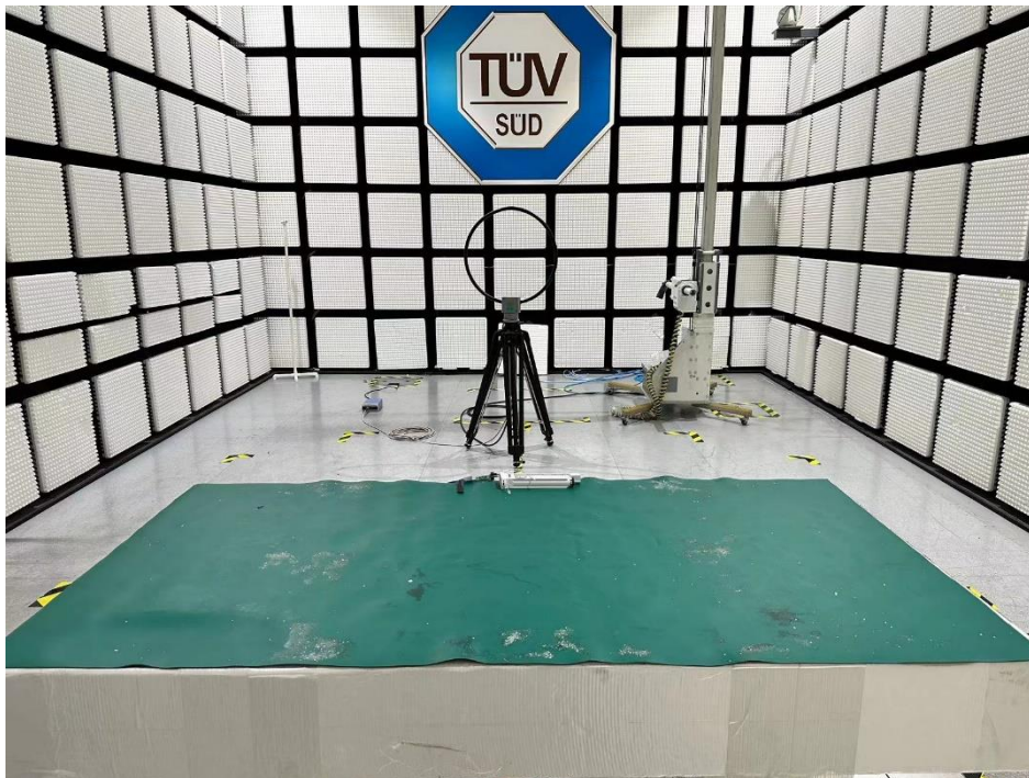
Radiated Emission Setup 9kHz ~ 30MHz
