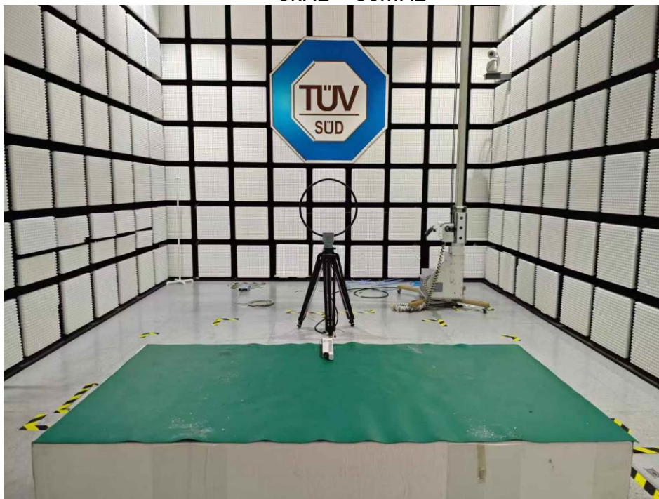
Radiated Emission Setup 9kHz ~ 30MHz
