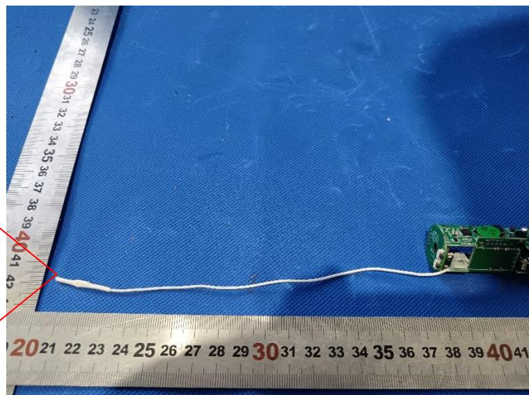
Antenna transmission frequency: 433.92MHz
