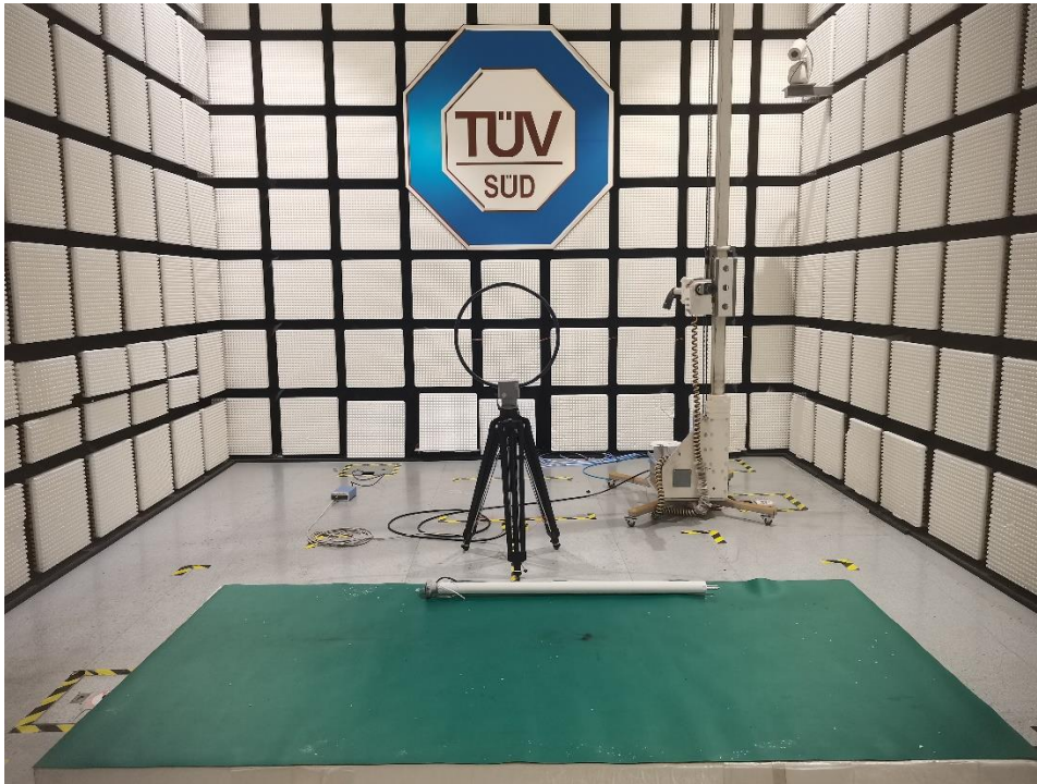
Radiated Emission Setup 9kHz ~ 30MHz
