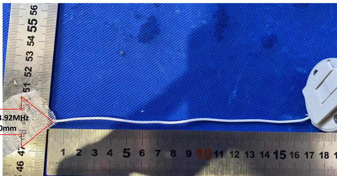
Antenna transmission frequency: 433.92MHz
