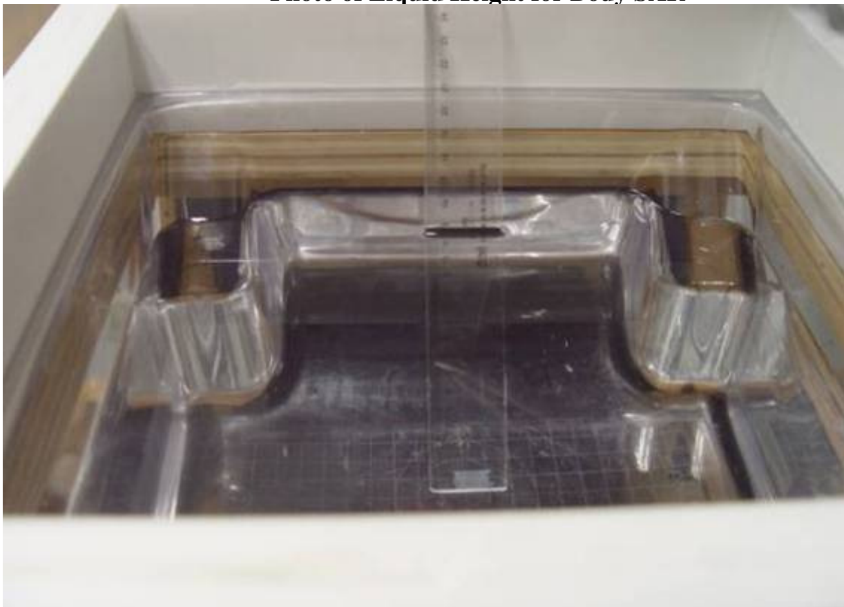
Photo of Liquid Height for Body SAR
