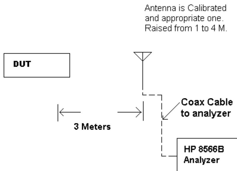
**METHOD OF MEASUREMENT:** The procedure used was ANSI standard C63.4-2003 & the FCC/OET Guidance on Measurements for Spread Spectrum Systems – KDB 558074 Dated March 23, 2005.
