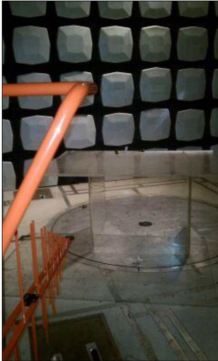
Photograph 2. Radiated Emissions, Test Setup
