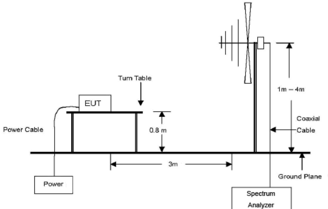
The diagram below shows the test setup that is utilized to make the measurements for emission from 1 GHz to 25 GHz Emissions.
