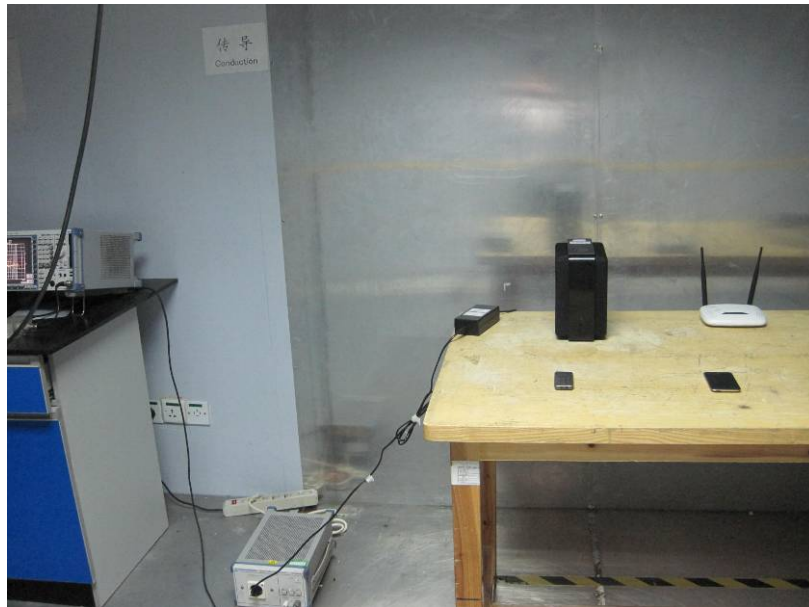
Photograph – Conducted Emission Test Setup
