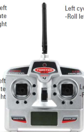
Each dual axis stick unit of your transmitter controls 2 helicopter functions (complete with trimmers on each function) giving you control about all 4 axes of flight). See above
