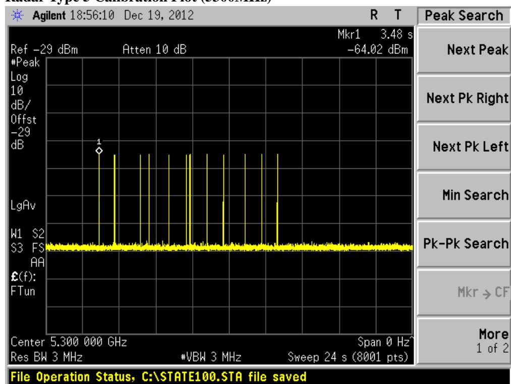
**Radar Type 5 Calibration Plot (5510MHz)**
