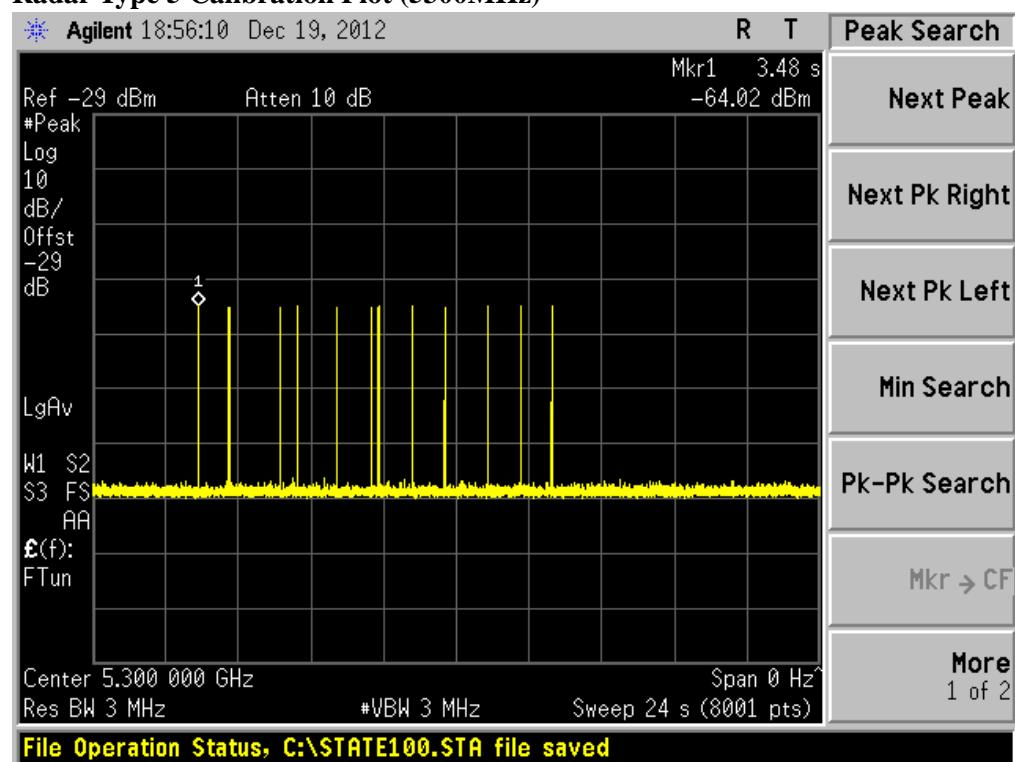
**Radar Type 5 Calibration Plot (5510MHz)**
